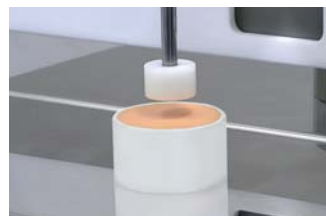
The sample material should be put in the vessel full to the brim.
