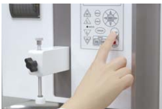
Set the sample material on the platform. Select Texture from the MENU and press START key.
