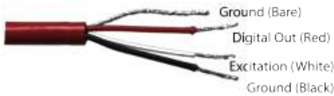
Figure 2: Pigtail End Wiring
